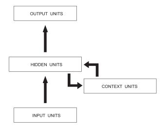
Fig. 1. Simple recurrent network. Each layer is composed of one or more units. Information flows from input to hidden to output layers. In addition, at every time step t, the hidden unit layer receives input from the context layer, which stores the hidden unit activations from time t - 1.
